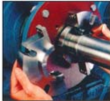
2. Place gland halves around rotary unit and fasten together.
