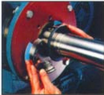
1. Position and secure rotary unit to shaft.
