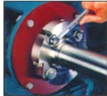
3. Bolt gland to pump. Connect flush if required.
